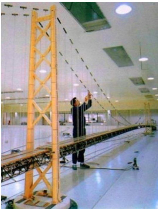
Akashi Kaikyō Bridge model in a wind tunnel
