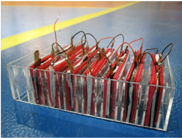
Fig. 6: Plexiglass MZAFC holder
